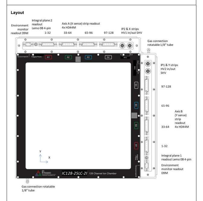
Designation of axes as X /Y, or horizontal / vertical is arbitrary, as it depends upon the orientation of the IC with respect to the beamline.
