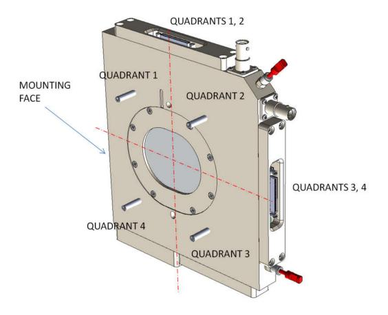
A beam entering the face shown passes through the anode then the cathode. The view of the cathode pixel pattern on the next page is looking through the face shown and through the anode.
