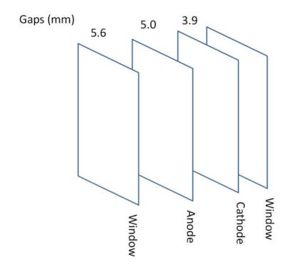
The sequence of layers corresponds to the illustration on the following page. Beam direction is arbitrary.
