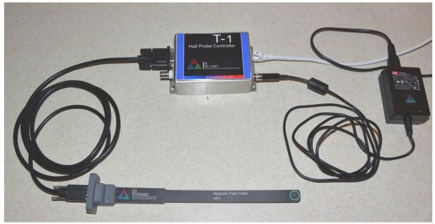
1) Find the cable that joins the T-1 to the HP-1 probe and connect each end. There is a standard 9-pin DSub connector on the T-1 and a micro D connector on the probe.
