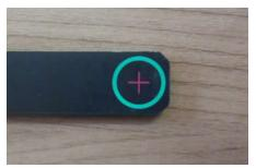
The field reading will be a positive value for a magnetic field vector entering the top surface of the probe, as shown below.
