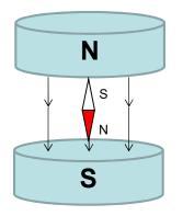
The HP-1 probe measures the field component that is perpendicular to the flat face of the probe, at the position of the red cross mark. If you orient the probe so that the field vectors point into the bulls eye, you will get a positive field reading, as shown below. The figure also shows the deflection direction of a positive ion beam for the illustrated field direction, and the conventional current direction in the coils of an electromagnet producing the field.
